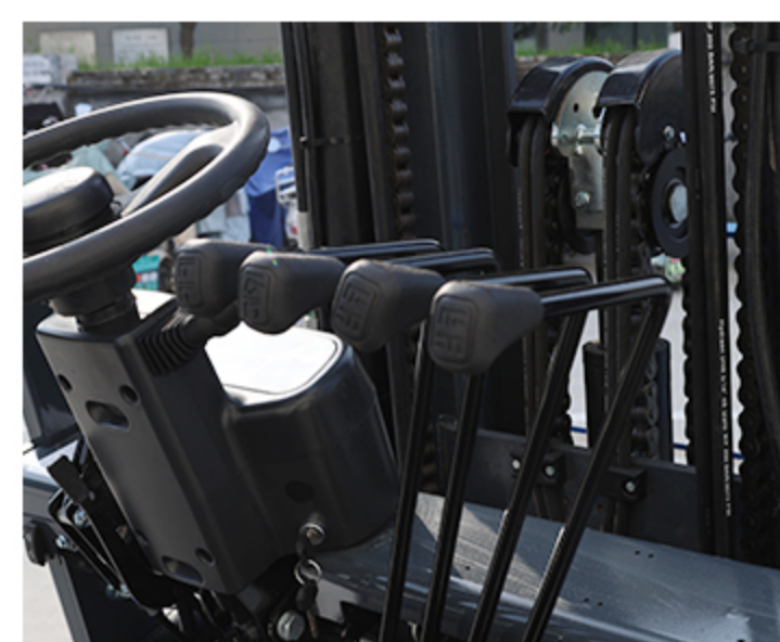
Control levers with contoured knobs for ease of control
