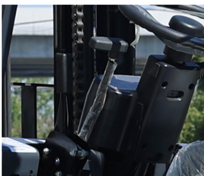
Finger-tip operation with the electric F/R lever
