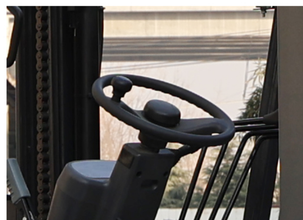
Finger-tip operation with the electric F/R lever
