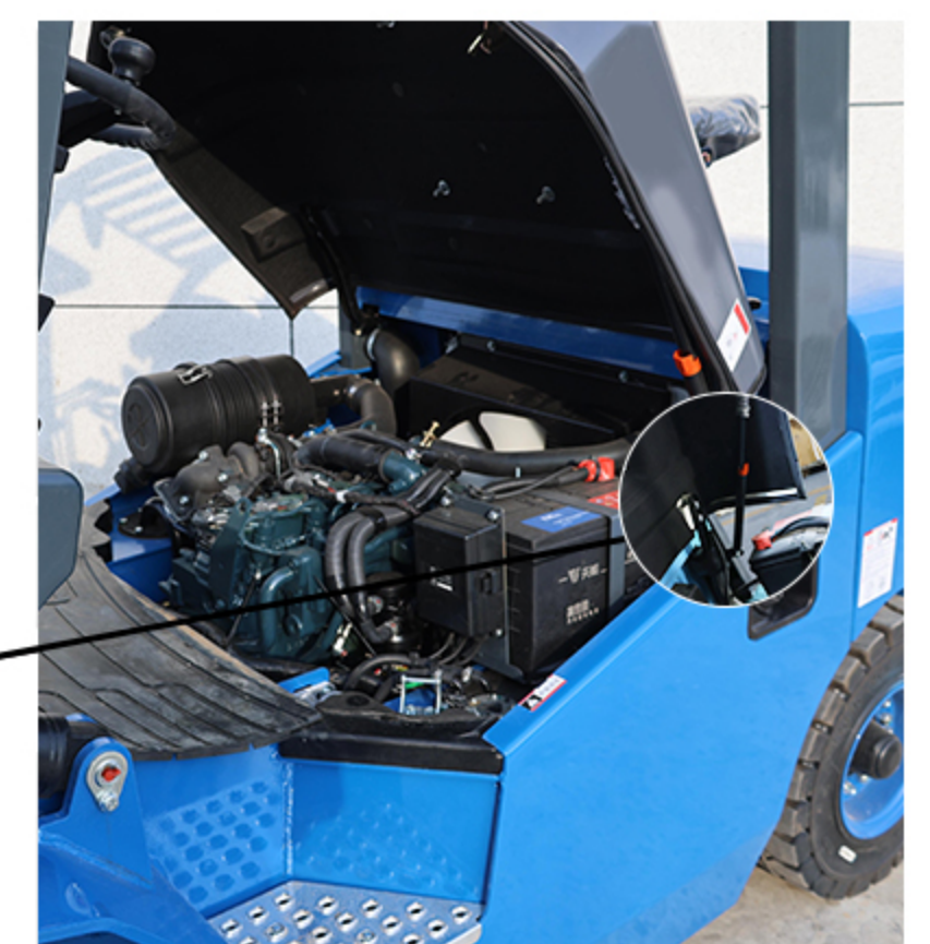
Locking engine hood provides protection while servicing
